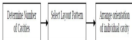
Fig 3: Automatic cavity layout design [4]
