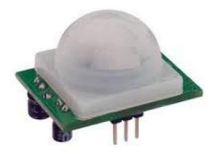
The PIR sensor is placed at the entrance so that it can detect human presence and during the night it can even set off a burglar alarm when required. The output of the PIR sensor is given to the PIC microcontroller and is interfaced accordingly.
