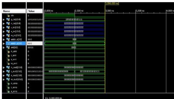
Fig 3: Data towards South Port with no Error
