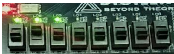
Fig.12. Implementation results for writing data to EEPROM (24C02)
