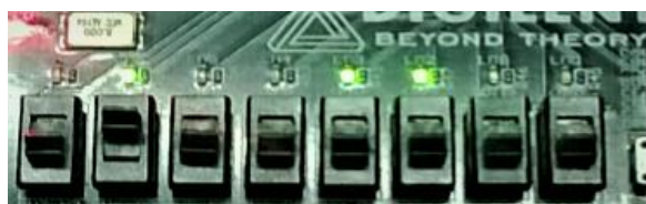
Fig.13. Implementation results for reading data from EEPROM (24C02).
